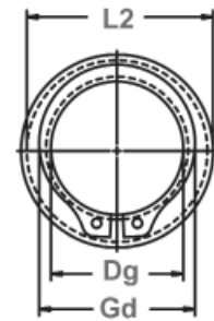
Clearance Diameter & Gaging Diameter Released in Groove.
