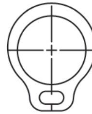
Alternate Lug Design For Sizes MSH-4 Thru MSH-6
